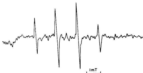
Fig. 1. ESR spectrum of the (DMPO–OH) ^{\cdot} adduct generated in dye 5 aqueous solution containing DMPO by irradiation for 15 min.
