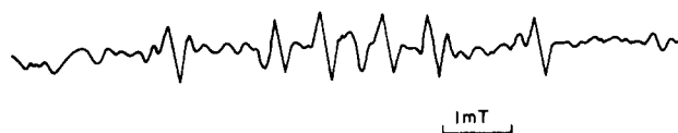
Fig. 5. ESR spectrum of the (DMPO-CH_3) adduct generated by irradiation of a solution ( H_2O:DMSO = 1:1 ) of dye 5 containing DMPO in a nitrogen atmosphere.
